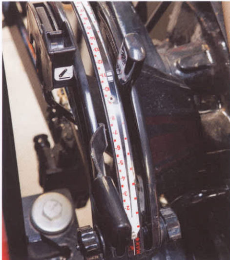
▼ Mechanical draft control MDC features Position, Draft and Mixed control.
